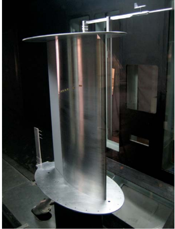
Figure 5: MACW model was tested at the Subsonic Aerodynamic Research Lab at the Wright Patterson Air Force Base (June 2006). Testing at the wind tunnel served to test the model and all aerodynamic instrumentation prior to flight testing.
